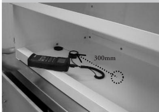
FIGURE 19. LIGHT INTENSITY TEST—PLACING THE PROBE 3
