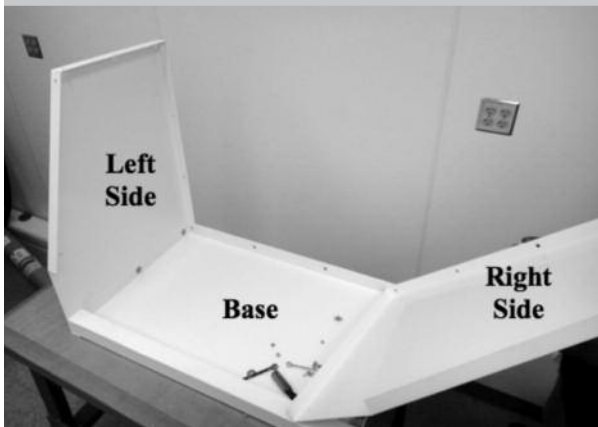
FIGURE 6. JOINING THE SIDES TO THE BASE
