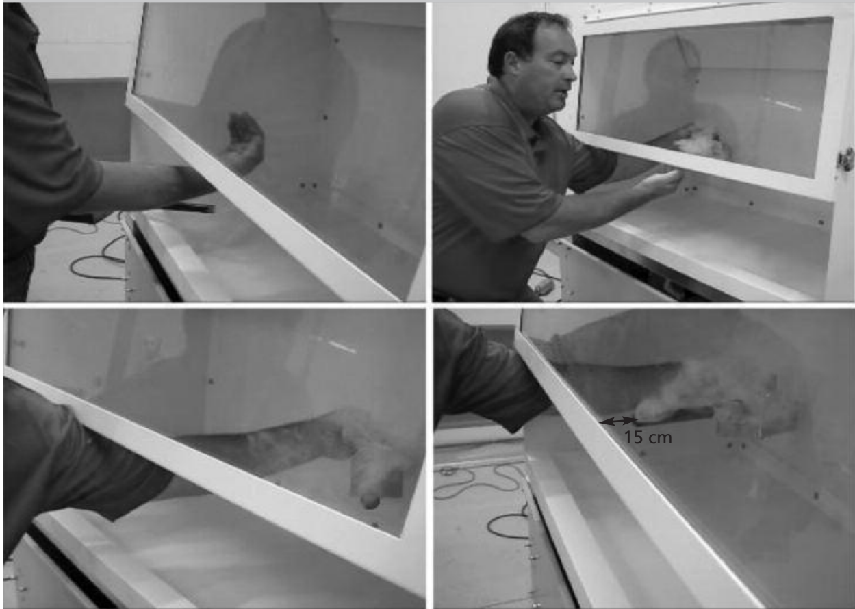
FIGURE 31. AIRFLOW SMOKE TEST – INTERNAL PERIMETER
