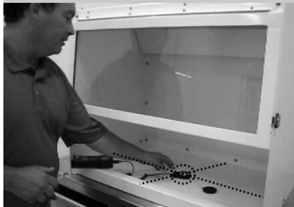
FIGURE 17. LIGHT INTENSITY TEST—PLACING THE PROBE 1
