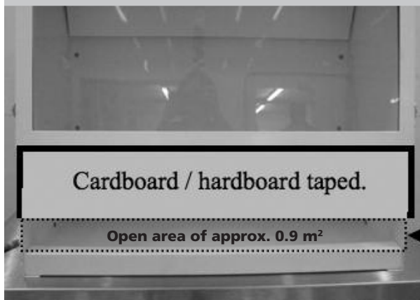
FIGURE 25. INWARD AIRFLOW TEST USING CARDBOARD INSERT
