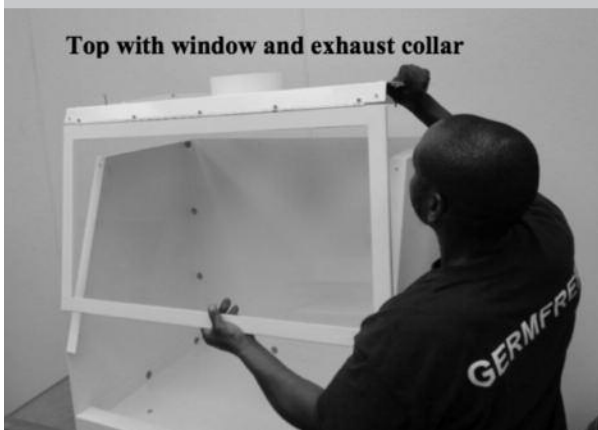
FIGURE 8. ATTACHING THE WINDOW
